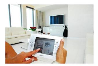
All audio, video, HVAC equipment, lighting, electrical blinds / curtains and other resources may be controlled locally from the room via a keypad, touch panel or remote control unit. One control procesor may be assigned for controlling several rooms. All control processors are networked. Information is passed to the central control system so the hotel personnel can view the status, take actions or just plan maintenance work in advance.
